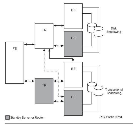
Figure 1–14 Two Sites: Transactional and Disk Shadowing with Standby Servers
